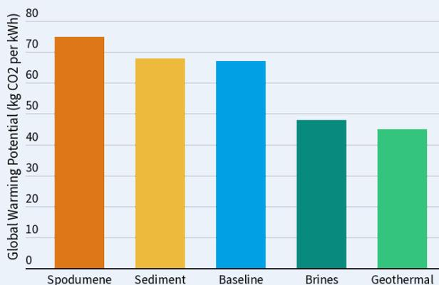
Impact for a Sulfide SSB (LFP Cathode)
