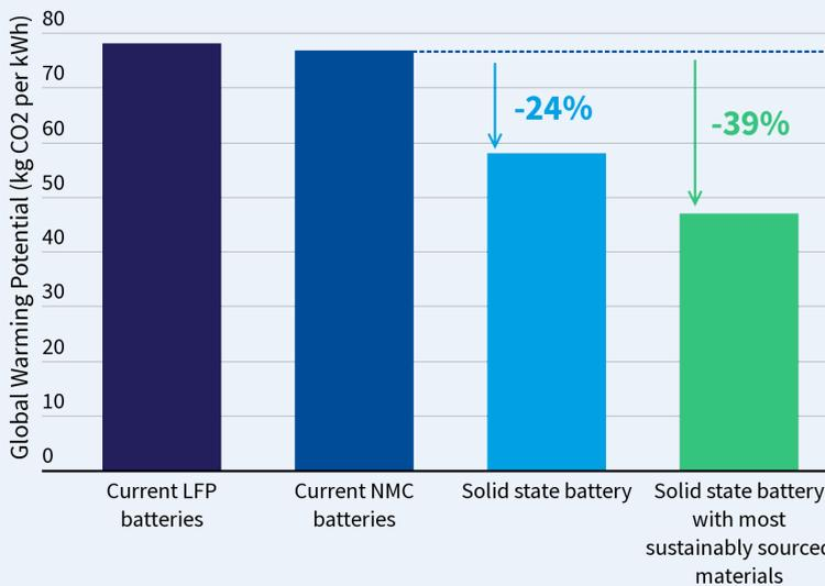
Results for displayed solid state batteries are with an oxide solid electrolyte and a NMC cathode
