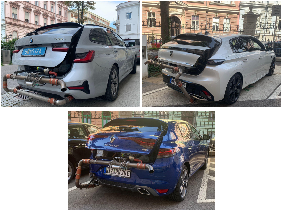
Fig. 1: The three PHEVs testest by TU Graz: BMW 3 xDrive series, Peugeot 308 and the Renault Megane with installed Portable Emission Measurement System.
